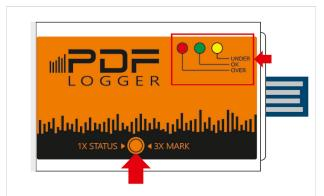
The alarm status of the activated and recorded device can be controlled by the LEDs on the Device.
