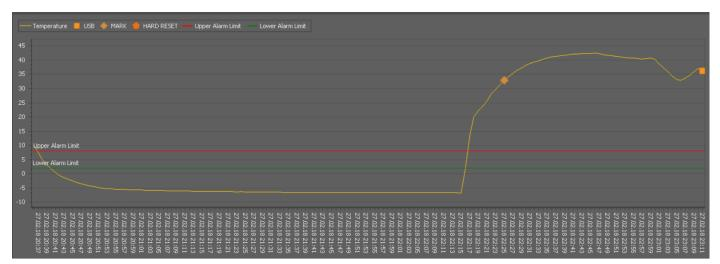
The data recorded on this screen is graphically displayed on the date Chart. If device is plugged into the USB before or end of shipment marks can be seen on this Screen.
